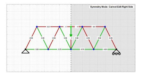
Angel's results from the truss analyzer program and the equations that were discussed in the introduction were as follows (these values were found by applying a 325 pound load at the apex of the truss):
