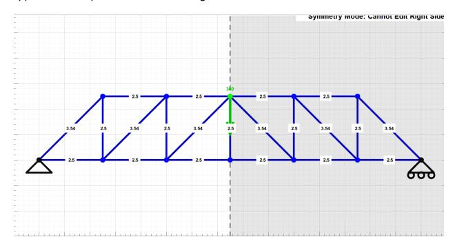
This is the final truss design, with member lengths.
